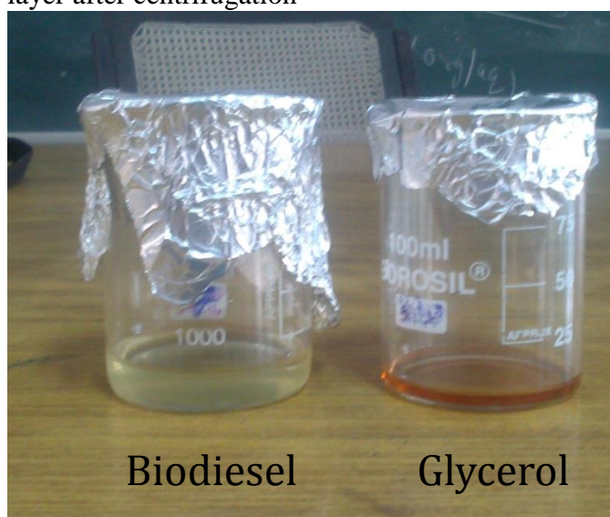
Figure 3: Separation of two distant layer of biodiesel and glycerol
