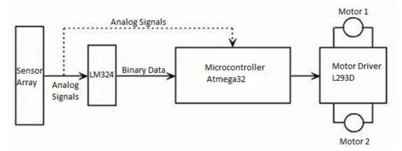
Figure 1. Block diagram of industrial fire fighting robot
