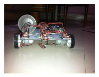
Figure 5: Fire fighting mobile robot
