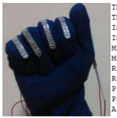
Thumb\_Resistance: 82000 ohms Thumb\_Bend: 6 degrees Index\_Resistance: 147000 ohms Index\_Bend: 117 degrees Middle\_Resistance: 169000 ohms Middle\_Bend: 132 degrees Ring\_Resistance: 155000 ohms Ring\_Bend: 126 degrees Pinkey\_Resistance: 97000 ohms Pinkey\_Bend: 107 degrees
