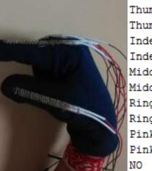
Thumb\_Resistance: 82000 ohms Thumb\_Bend: 6 degrees Index\_Resistance: 77000 ohms Index\_Bend: 4 degrees Middle\_Resistance: 92000 ohms Middle\_Bend: 8 degrees Ring\_Resistance: 155000 ohms Ring\_Bend: 126 degrees Pinkey\_Resistance: 97000 ohms Pinkey\_Bend: 107 degrees
